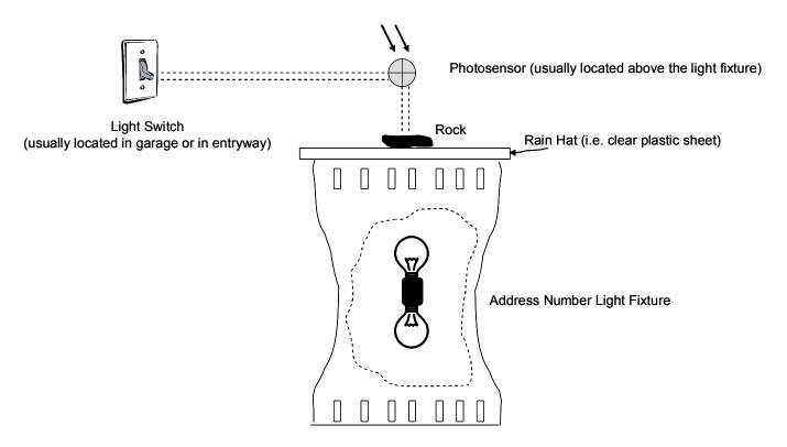
Note: While the typical installation is shown above, the following exceptions do occur: no light switch, no photosensor and/or only one light bulb
